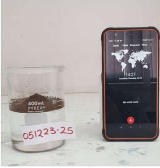
In conclusion, this absorbent material is not wetted by water and floats in it for a long time (at least 5 days).
